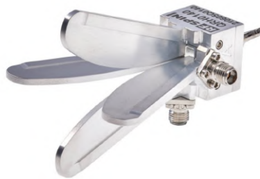
Figure 3.8: RF SPIN QRH0140 quad-ridged horn antenna [29].
