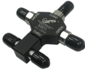
Figure 3.11: Copper Mountain S2611 coaxial SOLT calibration kit.
