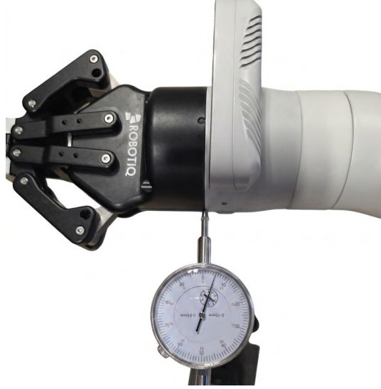
Figure 3.13: Dial test indicator setup used for robotic arm positioning accuracy characterisation.
