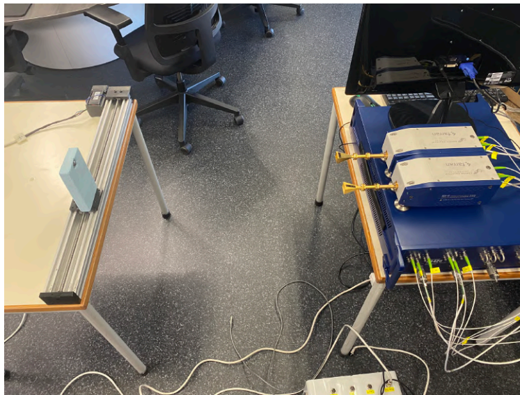
Figure 4.25: Experimental setup to analyse the influence of phase centre variation.
